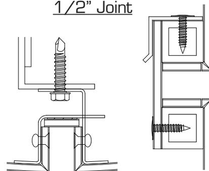
Our standard **COLUMN COVERS** are available with a hairline or a half inch wide joint with either a dry reveal, caulked, or silicone gasket. We offer MCM or .125 Aluminum Plate in a wide variety of colors and finishes. The newly redesigned attachment system ensures an easy installation and great fit of the column panels. Because of our unique interlocking hanging system, the column panels are easily removable as well.
