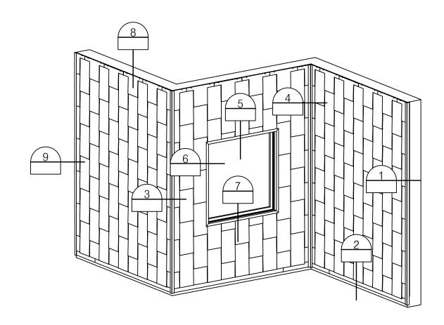
MAX-LOCKTM PANELS ARE AVAILABLE IN FOUR DIFFERENT WIDTHS: 12", 24", 30" AND 40"; AND TWO DIFFERENT HEIGHTS: 24" AND 30". THESE SIZES HAVE BEEN SELECTED TO MAXIMIZE YIELD FROM STOCK MCM SHEETS. FOR SIMPLICITY, WE ARE SHOWING THE 12 X 24 SIZE SHINGLE IN THE FOLLOWING DETAILS. DETAILS WILL BE SIMILAR FOR ALL SIZE SHINGLES, HOWEVER THE PATTERN PORPORTIONS SHOWN IN THE ISOMETRIC ABOVE WILL CHANGE. CONTACT MDSI FOR ADDITIONAL INFORMATION.
