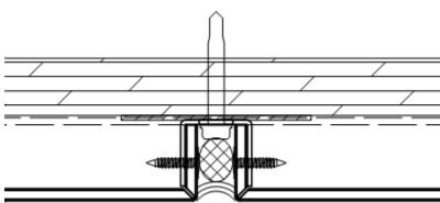
THE SERIES 10 is a simple rout and return, utilizing a staggered clip attachment which typically contains half inch wet sealed silicone joints. Series 10 is an economical system, easily applied to most fascia and soffit conditions, column covers and canopies.
