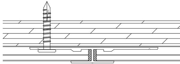
**THE SERIES 30** utilizes flat panels with an exposed trim attachment. This system is very cost effective and lends itself to be easily installed and modified in the field. Series 30 is typically specified when conditions call for a unique color brand or a radius application. It can be utilized in conjunction with our other systems to achieve a high polished look at an economical price.
