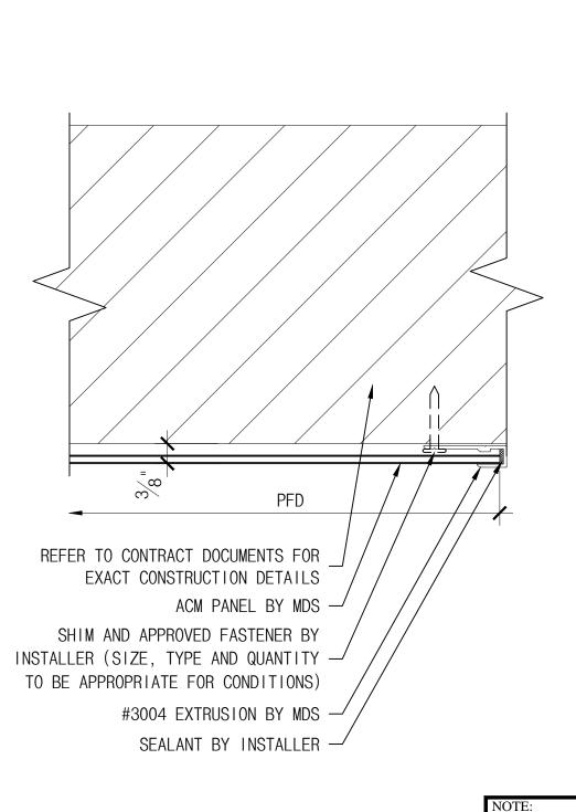
AIR/MOISTURE BARRIER INSTALLER MUST PROVIDE WEATHER TIGHT SEAL AT ALL BARRIER TERMINATIONS
