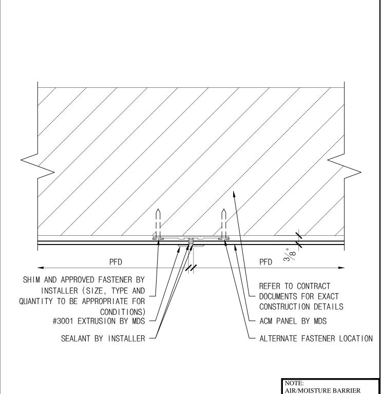
INSTALLER MUST PROVIDE WEATHER TIGHT SEAL AT ALL BARRIER TERMINATIONS
