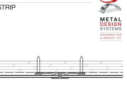
THE SERIES 30 utilizes flat panels with an exposed trim attachment. This system is very cost effective and lends itself to be easily installed and modified in the field. Series 30 is typically specified when conditions call for a unique color brand or a radius application. It can be utilized in conjunction with our other systems to achieve a high polished look at an economical price.
