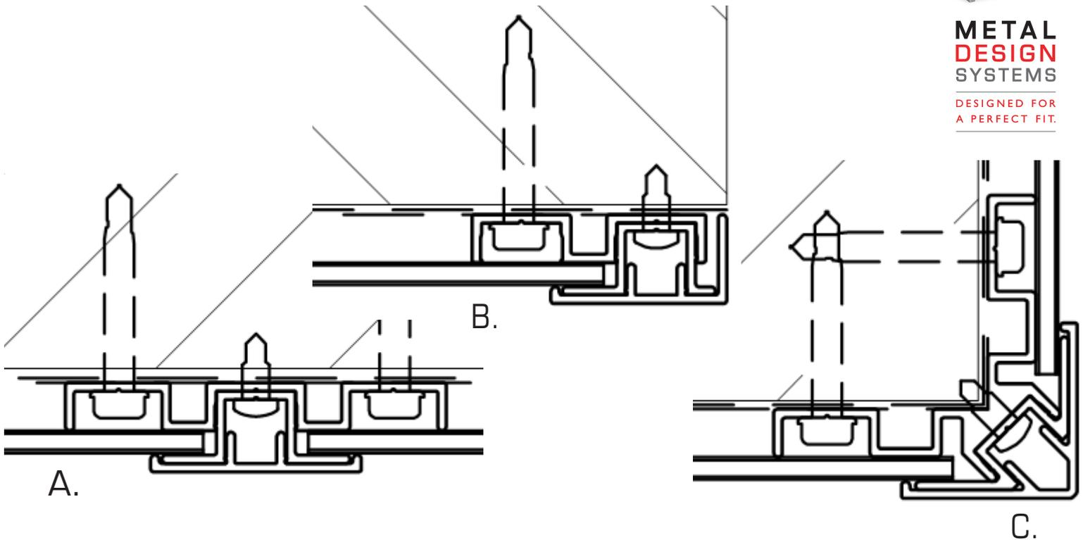
**Series 32** is a batten strip system where there are three extrusion types (pictured above), and each type has three pieces. The extrusion types are A: Joint, B: Perimeter, and C: Outside Corner. The pieces are base, retainer, and cover. The non-progressive install is very easy with flat ACM pieces sliding into the extrusions. This all aluminum batten system is an innovative interior or exterior option.
