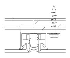
SERIES 40 is easy to install due to the semi-continuous attachment extrusions and the innovative lock-in-place backer wedge. This system is available as a wet sealed caulk system. Since the Series 40 is a non-progressive system, any panel can be removed or replaced without removing adjacent panels, further adding to the desirability of this system. Series 40, when installed offers clean lines, optimizes panel to panel alignment, and allows for thermal movement.
