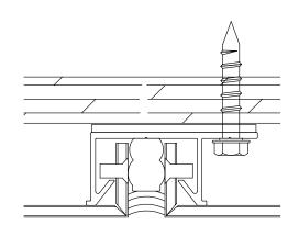
THE SERIES 40 is easy to intall due to the semi-continuous attachment extrusions and the innovative lock-in-place backer wedge. This system is available as a wet sealed caulk system. Since the Series 40 is a non-progressive system, any panel can be removed or replaced without removing adjacent panels, further adding to the desirability of this system. The Series 40 allows for thermal movement and when installed, it offers and holds clean lines and optimizes panel to panel alignment.
