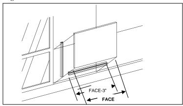
Note: The perimeter extrusion (#4001) can be installed in a continuous fashion. However, notches must be made in the extrusion where intersecting joints occur (Figure 14).
