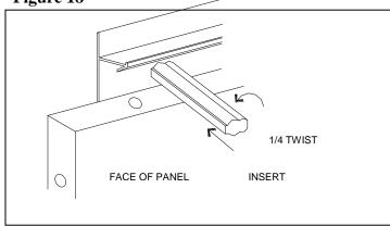
Insert the wedges about 3' on center but at least two on each edge. Do this to each edge that will have an adjoining panel.
