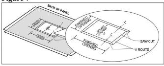
Use a fence to protect the good side of the panel and allow a clean straight rout (**Figure 8**).
