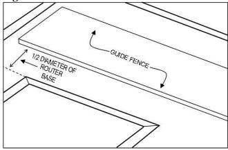
Two sided tape works well to temporarily secure the fence to the back of the panel (**Figure 9**).
