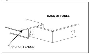
Locate the extrusion so that it is approximately 1 1/2" short of each end of the panel or centered on the length. Using one of the previously cut 6" lengths of plastic wedge, insert one end between the panel return and the hook of the aluminum extrusion and twist 90 degrees to lock the extrusion onto the panel (**Figure 18**).
