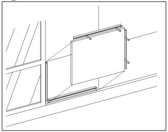
Loosely adjust the panel so that the alignment marks on the extrusion match up to the chalk lines on the wall. Using more of the 6" long wedges, insert them into the joint of the perimeter extrusion and the panel. These will be inserted to space the ½" wide joint so they will NOT be twisted (**Figure 20**).
