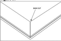
Back up the returns at the inside corners using a small piece of aluminum sheet bent to an angle. Pop-rivet or screw into place (**Figure 11**).
