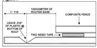
Saw cut the returns at the inside corners taking care not to cut past the v-rout (**Figure 10**).
