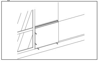
Make final adjustments to align the centerline marks and the layout lines and fasten extrusions to the wall. Drill clear holes in the extrusion at the witness groove that will align with the structural support framing. Fasten the extrusion to the wall using the appropriate fasteners and spacing (**Figure 15**). Metal Design Systems, Inc. recommends a minimum #12, 300 series stainless steel self-tapping fasteners for
