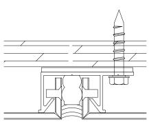
THE SERIES 40 is easy to intall due to the semi-continuous attachment extrusions and the innovative lock-in-place backer wedge. This system is available as a wet sealed caulk system. Since the Series 40 is a non-progressive system, any panel can be removed or replaced without removing adjacent panels, further adding to the desirability of this system. The Series 40 allows for thermal movement and when installed, it offers and holds clean lines and optimizes panel to panel alignment.
