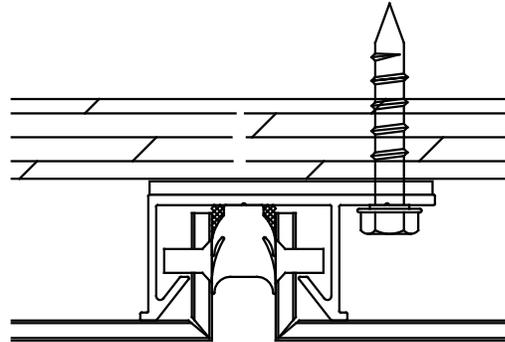
**THE SERIES 42** is easy to install due to the semi-continuous attachment extrusions and the innovative lock-in-place backer wedge. This system is available as a silicone gasket. Since the Series 42 is a non-progressive system, any panel can be removed or replaced without removing adjacent panels, further adding to the desirability of this system. The Series 42 allows for thermal movement and when installed, it offers and holds clean lines and optimizes panel to panel alignment.
