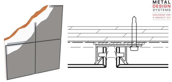
THE SERIES 42 is easy to intall due to the semi-continuous attachment extrusions and the innovative lock-in-place backer wedge. This system is available as a silicone gasket. Since the Series 42 is a non-progressive system, any panel can be removed or replaced without removing adjacent panels, further adding to the desirability of this system. The Series 42 allows for thermal movement and when installed, it offers and holds clean lines and optimizes panel to panel alignment.
