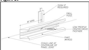
Metal Design Systems, Inc. recommends a minimum #12, 300 series stainless steel self-tapping fasteners for applications into steel or aluminum and #12, 300 series stainless steel T17 point fasteners for wood substrates. The recommended maximum spacing is 16" on center. Please reference the project specific details for fastener type and spacing requirements.
