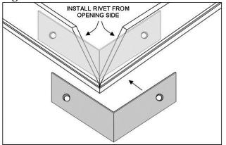
Back up the angle with butyl sealant (Figure 13).
