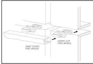
The clip should be started by hand and inserted as far as possible with hand pressure alone. Insert clip into the joint until it bottoms out on the aluminum extrusion and clicks into place. Clips shall be placed at 16"o.c. maximum and near each end of panels. The snap cover installs similarly (snapping into clip) locking the system into place (**Figure 24**).
