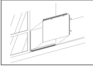
Loosely adjust the panel so that the alignment marks on the extrusion match up to the chalk lines on the wall. Using more of the 6" long wedges, insert them into the joint of the perimeter extrusion and the panel. These will be inserted to space the  $\frac{1}{2}$ " wide joint so they will NOT be twisted (**Figure 20**).
