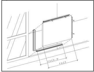
Note: The perimeter extrusion (#4401) can be installed in a continuous fashion. However, notches must be made in the extrusion where intersecting joints occur (Figure 15).
