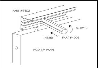
Insert the wedges about 3' on center but at least two on each edge. Do this to each edge that will have an adjoining panel.
