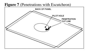
Note: If the object penetrating the panel does not have a weatherproof escutcheon, you will need to caulk around the object penetrating. Therefore the panel will require a return leg around the opening to caulk to. Cut opening in the same manner as above except that the opening should be 1" smaller than the object penetrating the panel. Using the router and the v-bit, rout grooves around the opening 1" away from the opening (Figure 8).
