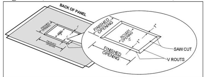
Use a fence to protect the good side of the panel and allow a clean straight rout (Figure 9).
