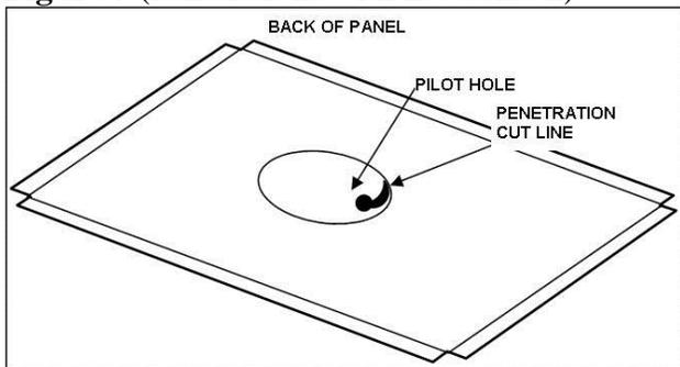
**Note:** If the object penetrating the panel does not have a weatherproof escutcheon, you will need to caulk around the object penetrating. Therefore the panel will require a return leg around the opening to caulk to. Cut opening in the same manner as above except that the opening should be 1" smaller than the object penetrating the panel. Using the router and the v-bit, rout grooves around the opening 1" away from the opening (Figure 8).
