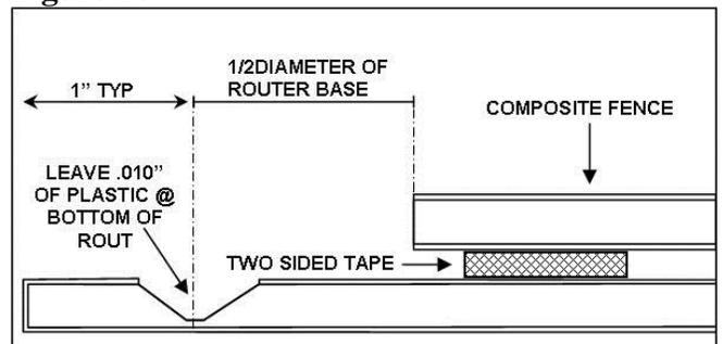
Saw cut the returns at the inside corners taking care not to cut past the v-rout (Figure 11).
