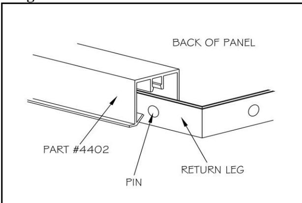
Locate the extrusion so that it is approximately 1 1/2” short of each end of the panel or centered on the length. Using one of the previously cut 6” lengths of plastic wedge, insert one end between the panel return and the hook of the aluminum extrusion and twist 90 degrees to lock the extrusion onto the panel (Figure 18).
