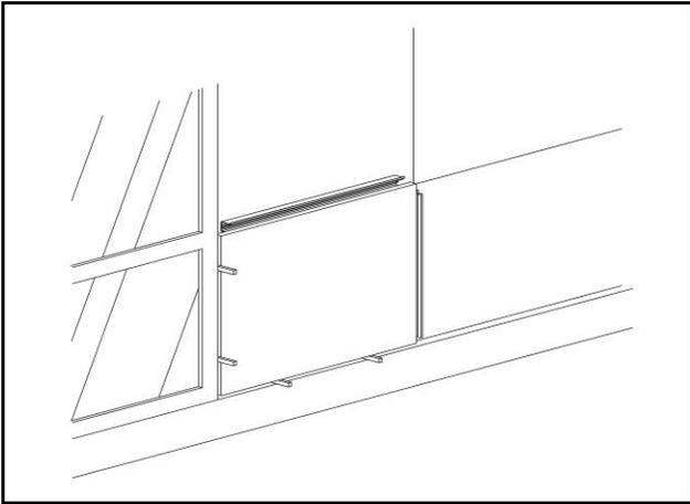
Make final adjustments to align the centerline marks and the layout lines and fasten extrusions to the wall. Drill clear holes in the center of extrusion that will align with the structural support framing. Fasten the extrusion to the wall using the appropriate fasteners and spacing (**Figure 21**).
