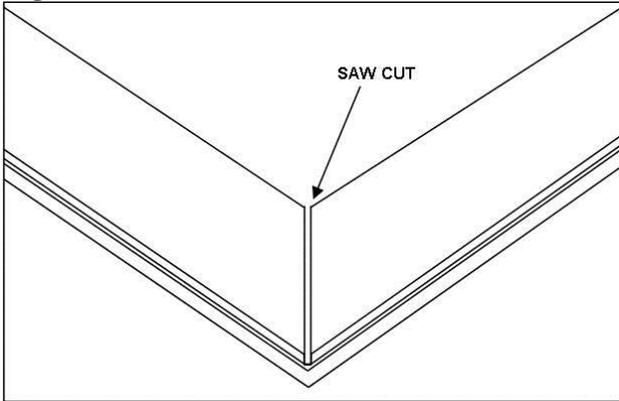
Back up the returns at the inside corners using a small piece of aluminum sheet bent to an angle. Pop-riquet or screw into place (**Figure 12**).
