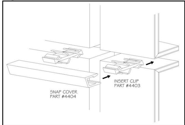
The clip should be started by hand and inserted as far as possible with hand pressure alone. Insert clip into the joint until it bottoms out on the aluminum extrusion and clicks into place. Clips shall be placed at 16" o.c. maximum and near each end of panels. The snap cover installs
