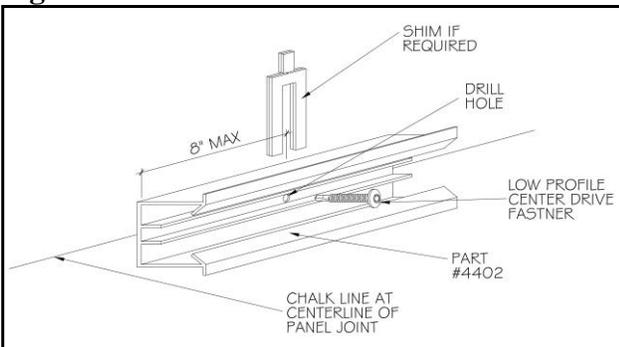
Metal Design Systems, Inc. recommends a minimum #12, 300 series stainless steel self-tapping fasteners for applications into steel or aluminum and #12, 300 series stainless steel T17 point fasteners for wood substrates. The recommended maximum spacing is 16" on center. Please reference the project specific details for fastener type and spacing requirements.
