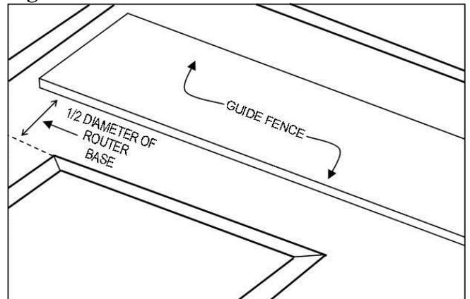
Two sided tape works well to temporarily secure the fence to the back of the panel (Figure 10).
