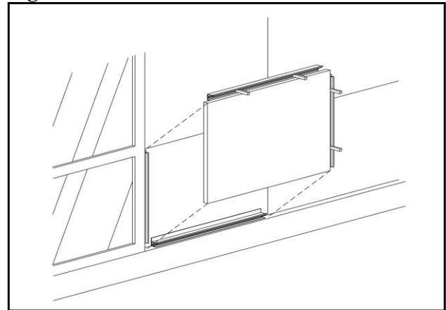
Loosely adjust the panel so that the alignment marks on the extrusion match up to the chalk lines on the wall. Using more of the 6” long wedges, insert them into the joint of the perimeter extrusion and the panel. These will be inserted to space the 1/2” wide joint so they will NOT be twisted (Figure 20).
