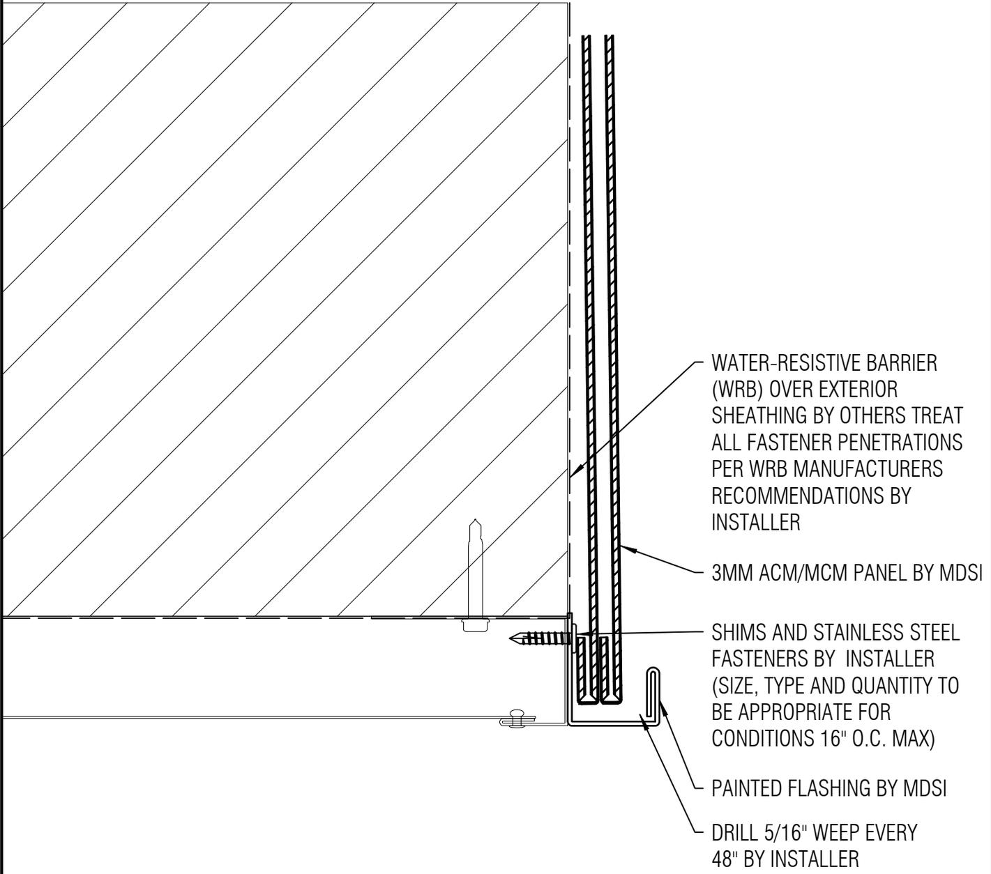
WATER-RESISTIVE BARRIER (WRB) OVER EXTERIOR SHEATHING BY OTHERS TREAT ALL FASTENER PENETRATIONS PER WRB MANUFACTURERS RECOMMENDATIONS BY INSTALLER
