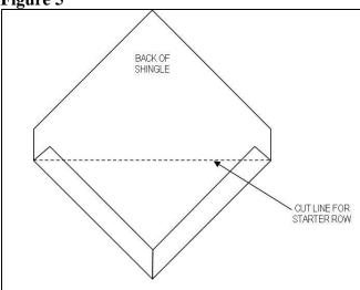
Remove the protective vinyl and install the starter row by placing the bottom straight edge of the flat, half cut shingles into the J channel and run a clip with fasteners into each side of the top of shingle. Butt each consecutive half shingle next to the previous one, working horizontally, until the starter row has been completed. Snap a vertical chalk line at every 3<sup>rd</sup> panel seam, making sure the lines are plum. This will help to control shingle
