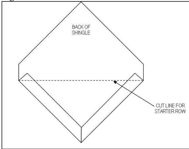
Remove the protective vinyl and install the starter row by placing the bottom straight edge of the flat, half cut shingles into the J channel and run a clip with fasteners into each side of the top of shingle. Butt each consecutive half shingle next to the previous one, working horizontally, until the starter row has been completed. Snap a vertical chalk line at every 3<sup>rd</sup> panel seam, making sure the lines are plum. This will help to control shingle
