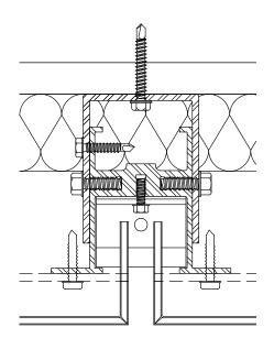
THE SERIES 70 is a hook and pin style system with no caulk or silicone and virtually maintenance free. This panel system features a continuous vertical channel with adjustable panel support pins. The panel returns are notched to hook over the support pins. This completed system is very clean and attractive.
