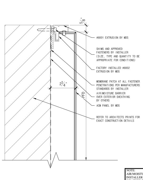
AIR/MOISTURE BARRIER INSTALLER MUST PROVIDE WEATHER TIGHT SEAL AT ALL BARRIER TERMINATIONS
